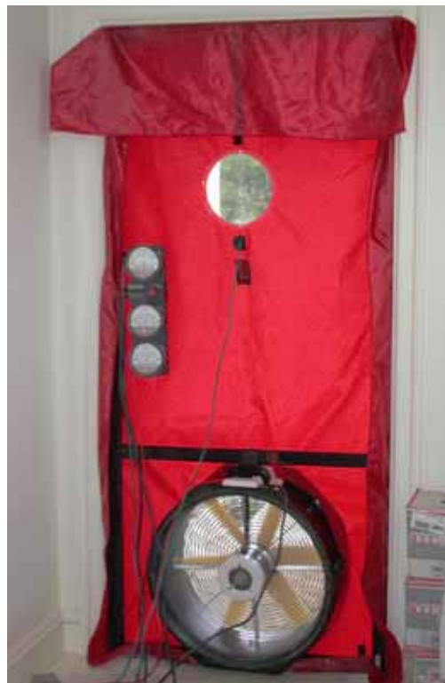
ABOVE: The blower door can be used in conjunction with the infrared camera and smoke pen, to locate points of moisture and air infiltration.
